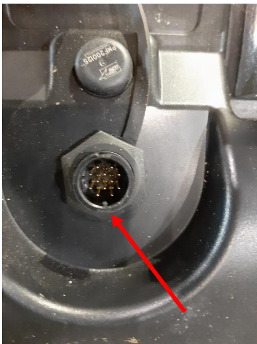
Figure 2 Connector of Locator One (red arrow)
