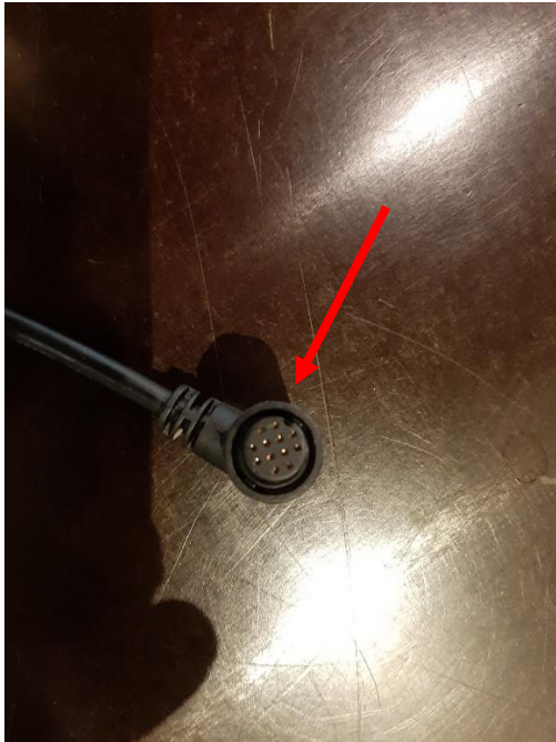
Figure 1 Notch of the 12-pins connector of the cable (red arrow)
